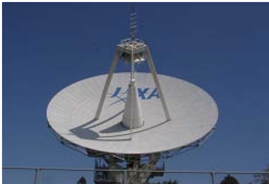
A 18m diameter antenna (JAXA Katsuura station)
