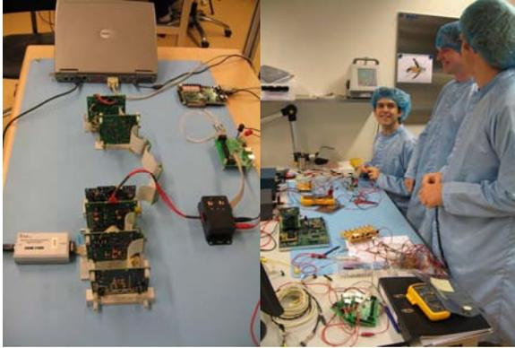
Figure 9: Delfi-C<sup>3</sup> subsystem tests in clean room
