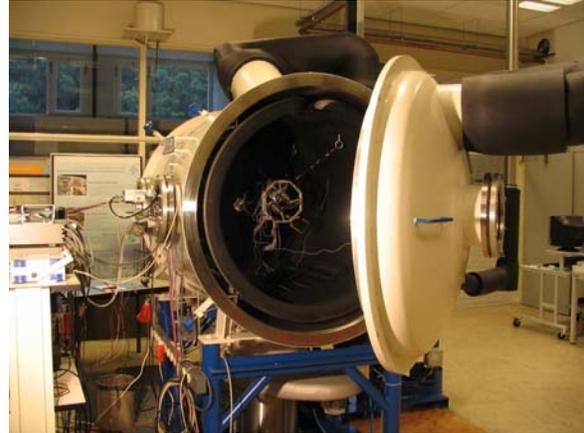
Figure 8: Delfi-C<sup>3</sup> in thermal vacuum chamber
