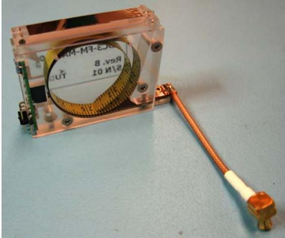
Figure 5: Antenna box side view
