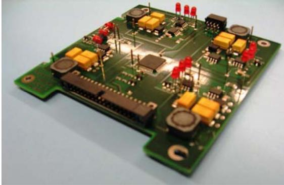
Figure 6: Electrical Power Subsystem PCB
