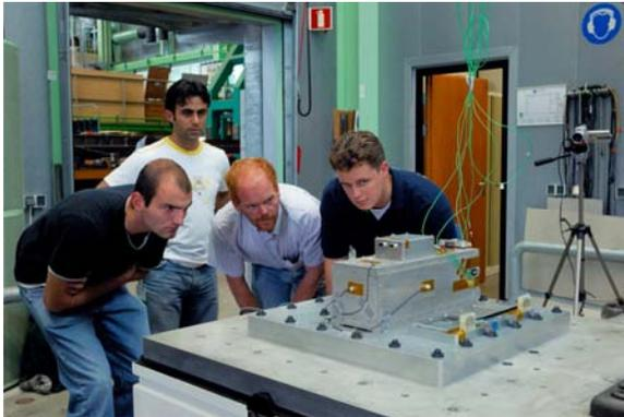
Figure 7: Vibration test on shaker table
