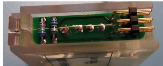
Figure 4: Antenna box deployment mechanism
